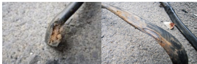
Break due to underwater cable twisting phenomenon
